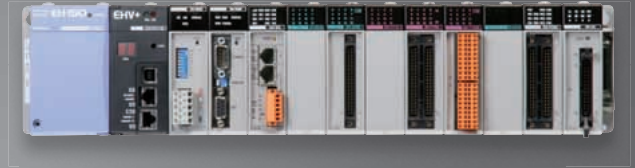
EH-150 system incl. EHV+ CPU and various I/O modules
