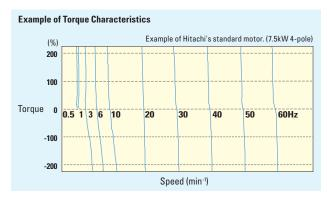
Speed regulation at low-speed is greatly improved. – Fluctuation is 1/2\* compared with the previous model. –
